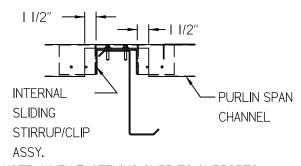
NOTE: WHEN FASTENING CURB TO SUPPORTS, OR WHEN FASTENING PANELS TO CURB, FASTENERS MUST BE KEPT I I/2" FROM PURLIN TO PREVENT LOCKING DOWN THE FLOATING CURB.
